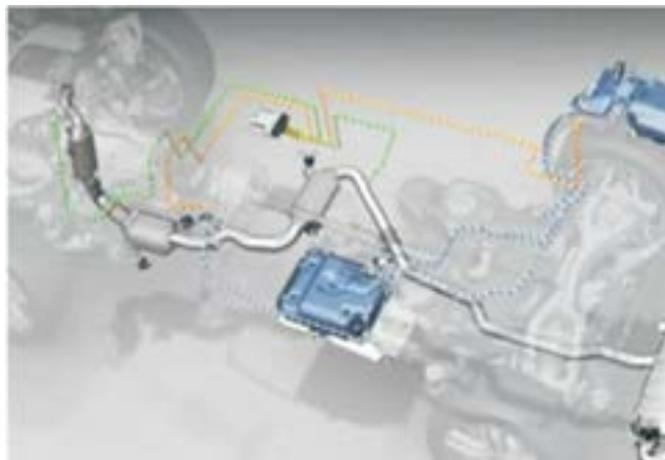
**Fig. 5.b.** The organisation of the post-treatment system of exhaust fumes for Audi Q7
