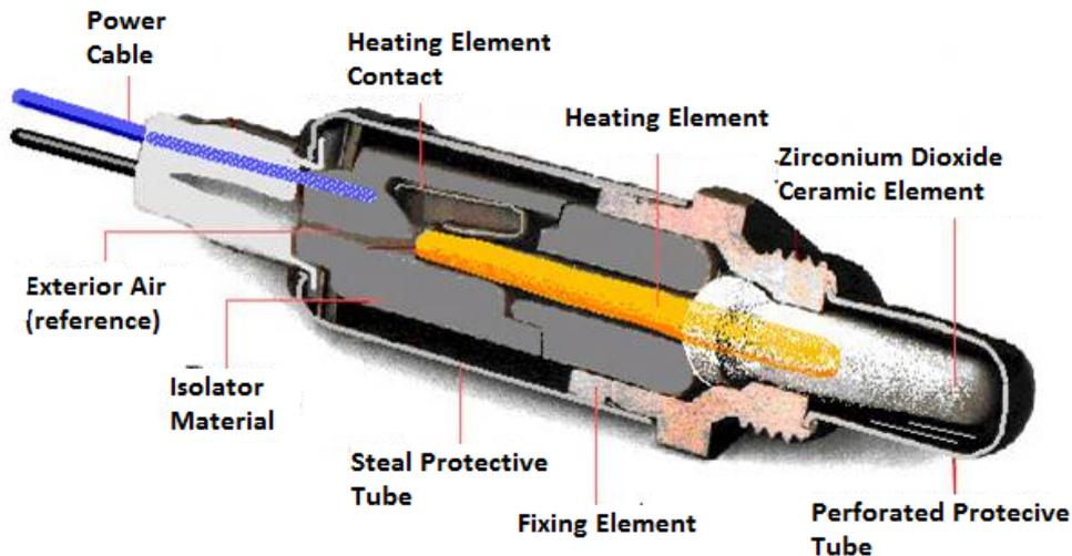
**Fig. 4.** Self-heating lambda sensor
